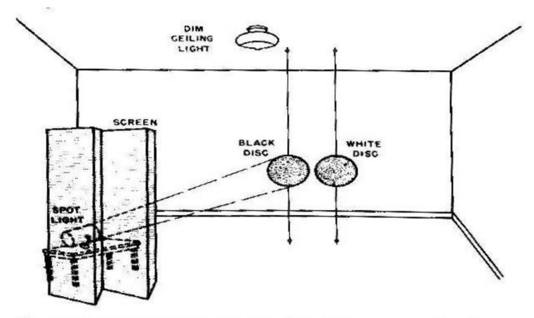
Fig. 12. Concealed illumination experiment. The person who does not know about the spotlight will judge the black and the white discs to have equal brightness. A small piece of paper thrust into the light beam, however, makes it obvious that the left disc is black.
